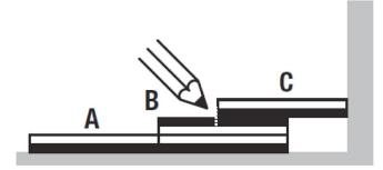
Now indicate on Tile B where you have to cut. Finally, install the cut Tile B in the space between the wall and Tile A.
